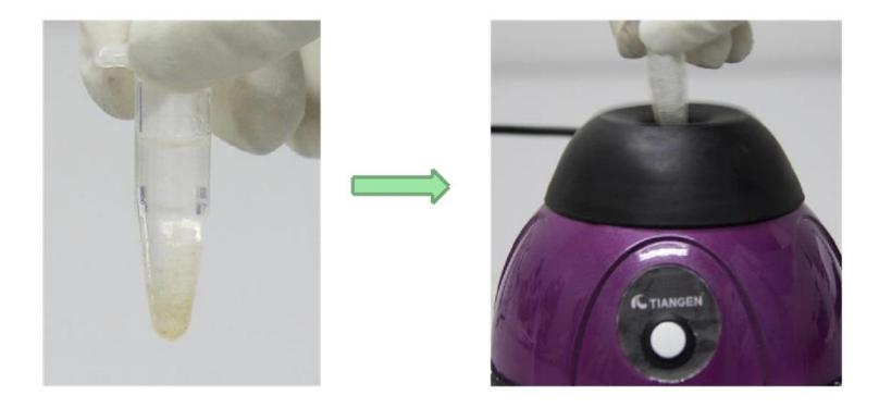
Place the sample in a 1.5 ml sterile centrifuge tube, add 1ml xylene, and vortex violently for 10 sec.
