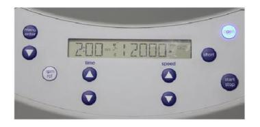
Centrifuge at 12,000 rpm (~13,400 g) at room temperature for 2 min, discard supernatant.
