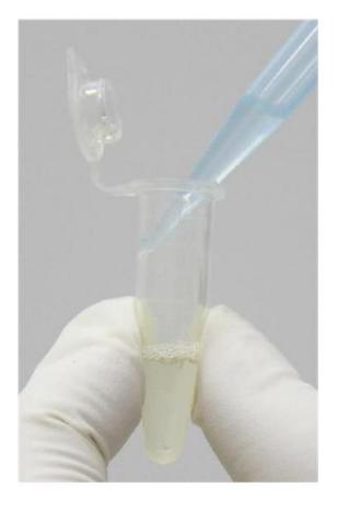
Add 220 µl Buffer GB, mix well by vortex. Add 250 µl 96-100% ethanol, vortex to mix thoroughly.
