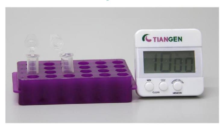
Place at room temperature for 5-10 min to fully volatilize ethanol.
