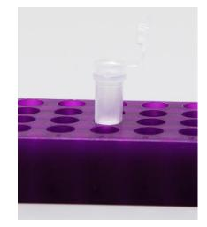
Centrifuge at 12,000 rpm ( $\sim$ 13,400 $\times$ g) for 2 min, and discard the waste liquid.
