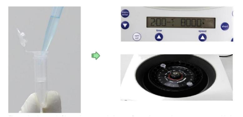
Transfer the solution and flocculent precipitate from the previous step to Spin Column CR2.Centrifuge at 8,000 rpm ( $\sim$ 6,000×g) at room temperature for 2 min, discard the waste liquid in the collection tube and place the Spin Column CR2 into the collection tube.
