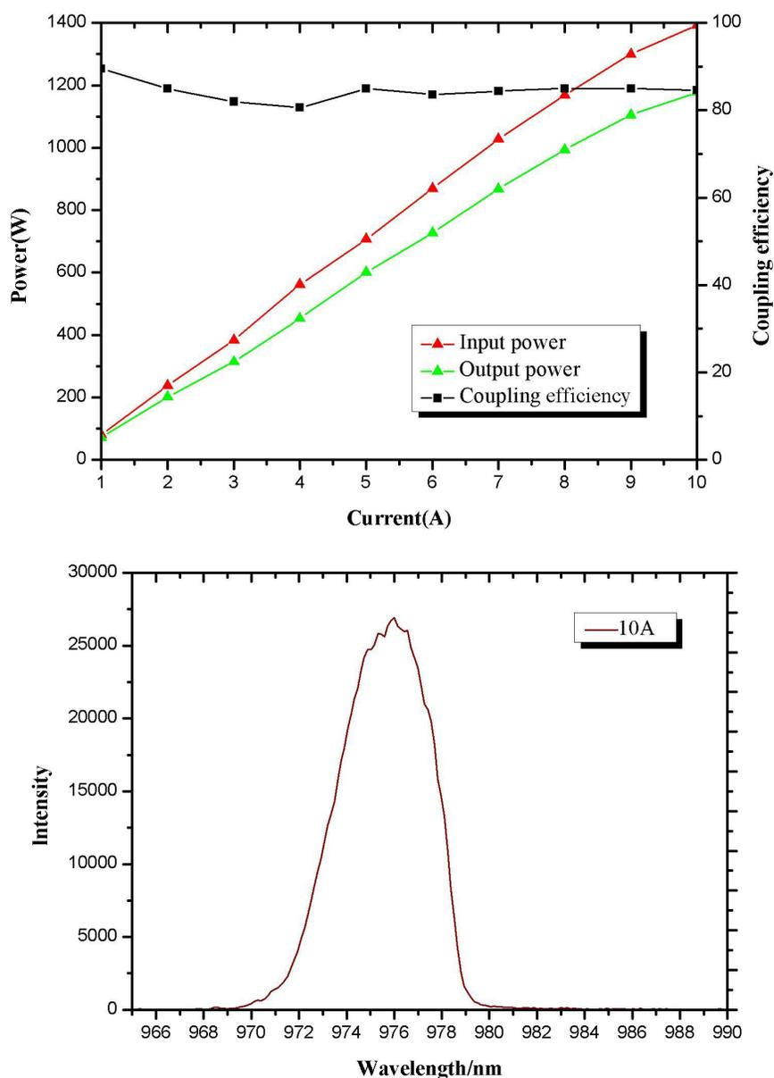
Figure 5. Coupling efficiency and spectrum.
