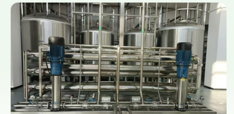
Reverse Osmosis Concentrated Water Filtration Unit of Hunan Kelun
